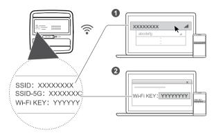
Once the router has connected to a mobile data network, you can connect your computer or mobile phone to the router's Wi-Fi network to access the Internet. Please refer to the label on the bottom of the router for the default wireless network name (SSID) and password (Wi-Fi KEY).
